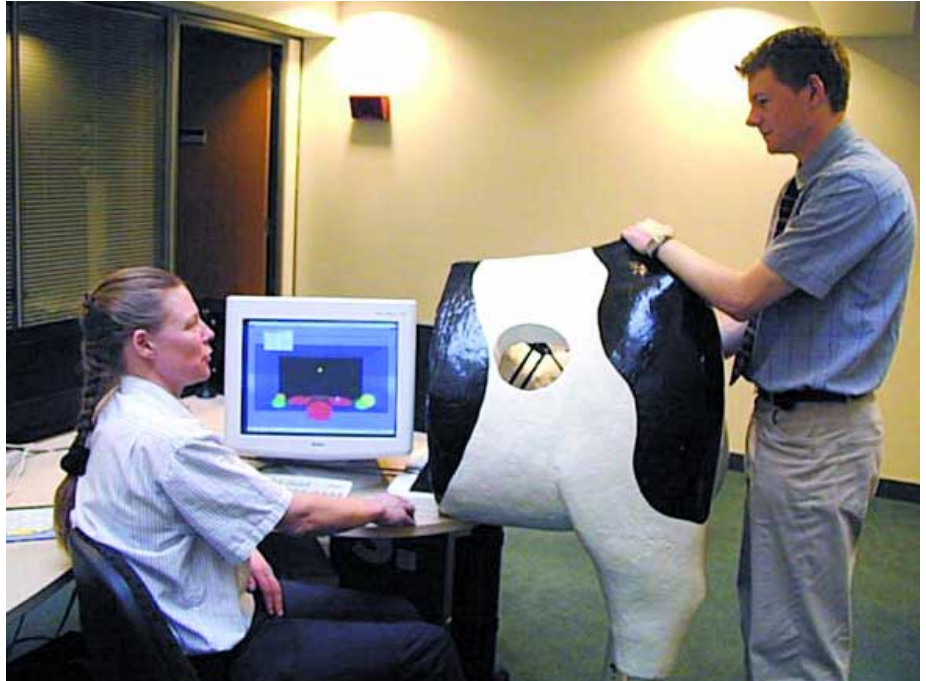
Figure 1 - a training session. The student palpates the virtual models of the bovine reproductive tract, interacting with the PHANTOM haptic device inside the fibreglass model cow, while the teacher follows the movements inside the cow on the screen and provides guidance (image used with permission).
